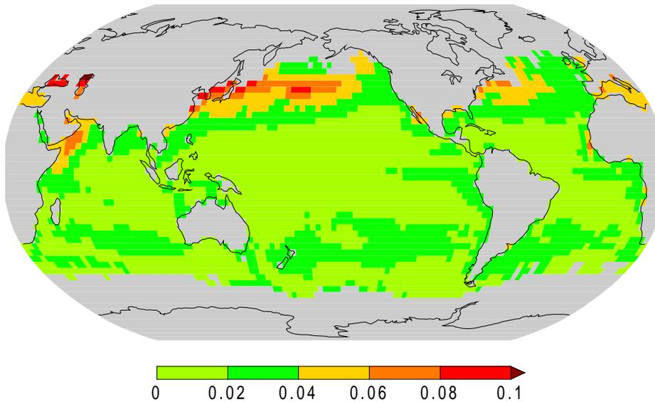
**Fig. 4b:** The actual reduction in the RMS error in daily temperature, which is achieved using the "new" method in comparison to the "traditional" method. See text for further explanation. (Units: K)
