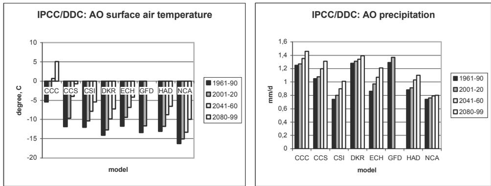
**Figure 4.** IPCC DDC AOGCM annual mean surface air temperature (left) and precipitation (right) over the Arctic Ocean region within  $70^{\circ}\text{N}$  (ocean only) simulated under GHG-only increase (IS92a scenario) – for different time slices. The projected changes, at least by the mid-21<sup>st</sup> century, are generally smaller than the across-model scatter of the present day values.
